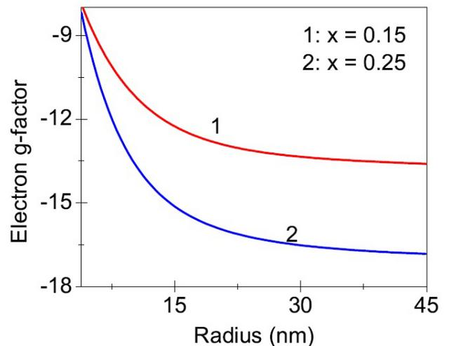
FIGURE 2. (Color online) Variation of the electron  $g$ -factor as a function of the radius in a GaSb/Ga<sub>1-x</sub>In<sub>x</sub>As<sub>y</sub>Sb<sub>1-y</sub>/GaSb SQD at  $T=300$  K. Lines 1 and 2 corresponds for  $x=0.15$  and  $x=0.25$  respectively.
