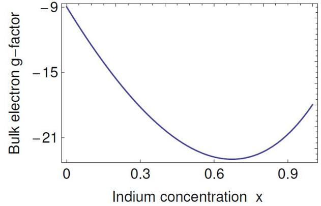
FIGURE 1. (Color online) Bulk electron  $g$ -factor as a function of  $x$ , for Ga<sub>1-x</sub>In<sub>x</sub>As<sub>y</sub>Sb<sub>1-y</sub>/GaSb quaternary alloys at  $T=300$  K.
