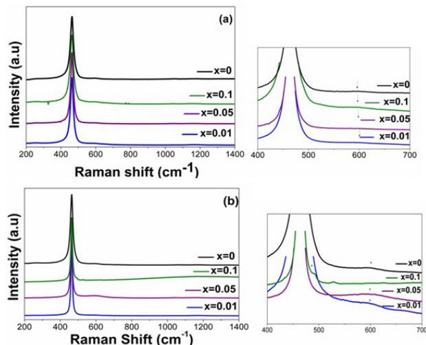
FIGURE 2. Raman spectra of  $Ce_{1-2x}Zn_xCo_xO_{2-\delta}$  with variation of  $x = 0, 0.01, 0.05$  and  $0.1$  for samples calcinated at (a) 600 and (b) 800°C.
