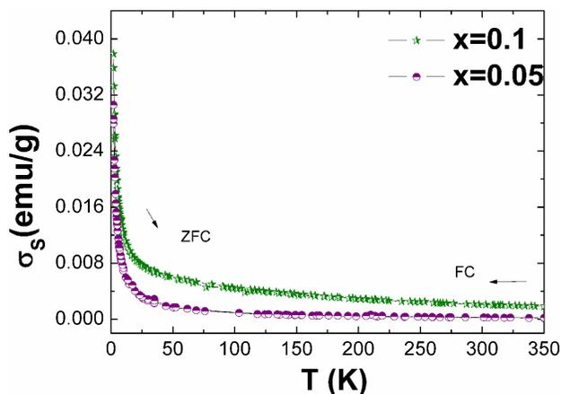
FIGURE 4. Magnetization versus temperature (ZFC and FC) for  $Ce_{1-2x}Zn_xCo_xO_{2-\delta}$  with variation of  $x = 0.1$  and  $0.05$  for samples calcined at  $800^\circ C$ .
