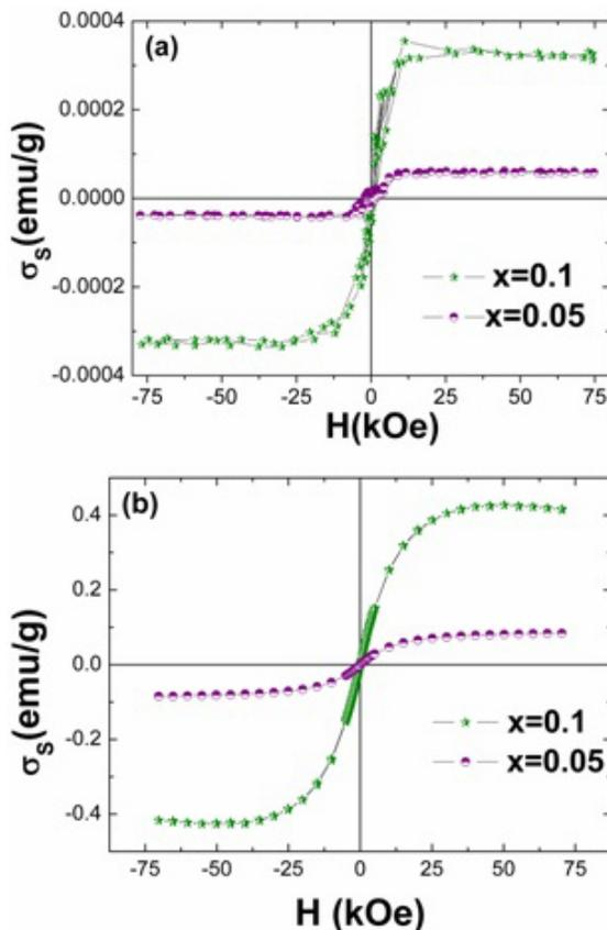
FIGURE 3. Magnetization loop at (a) 2 and (b) 300 K for  $Ce_{1-2x}Zn_xCo_xO_{2-\delta}$  with variation of  $x = 0.1$  and  $0.05$  for samples calcinated at 800°C.
