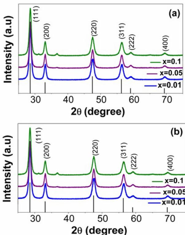
FIGURE 1. XRD patterns recorded at room temperature for samples  $Ce_{1-2x}Zn_xCo_xO_{2-\delta}$  prepared at (a) 600°C and (b) 800°C with varying dopant concentrations. The expected peak positions are indicated for  $CeO_2$  along the x-axis.
