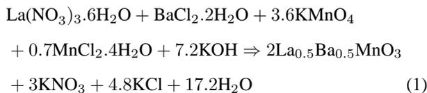
The product is poured into the Teflon container with a filling factor of 60%, this is set in an autoclave and heated to 240°C for 24 hours. The final compound is washed with distilled water several times, finally dried at 80°C. The product (brown powder) is carried to a furnace and heated to a series of ramps up to the final temperature of 1000°C.
