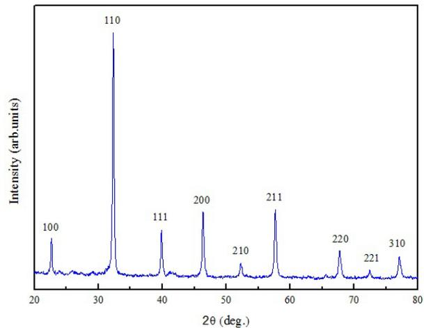
FIGURE 1. X-ray diffraction at room temperature for  $\text{La}_{0.5}\text{Ba}_{0.5}\text{MnO}_3$ . Miller indices are assigned to a cubic structure.
