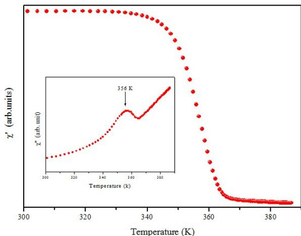
FIGURE 3. Real part of AC susceptibility, depending on the La<sub>0.5</sub>Ba<sub>0.5</sub>MnO<sub>3</sub> temperature, for a frequency of 95 kHz. The inset shows the AC susceptibility imaginary part. The transition temperature  $T_c = 356$  K
