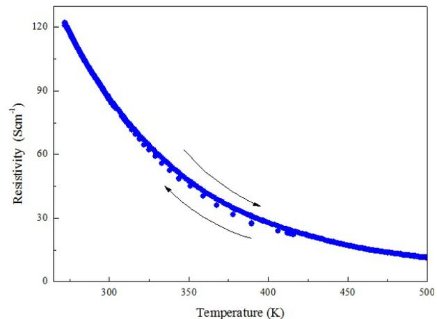
FIGURE 2. Resistivity variation with the temperature for LBMO. The arrows indicate the direction of heating or cooling.
