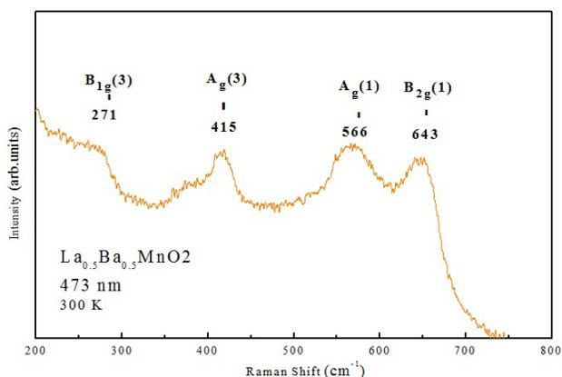
FIGURE 4. La<sub>0.5</sub>Ba<sub>0.5</sub>MnO<sub>3</sub> Micro-Raman spectrum compound at room temperature.
