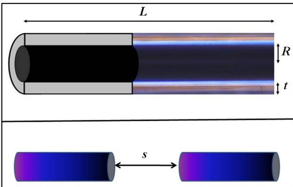
FIGURE 1. (Top) Schematic of the coated microwire contrasted with a phase contrast microscopy image of the  $\text{Fe}_{77.5}\text{Si}_{7.5}\text{B}_{15}$  amorphous sample. (Bottom) Axially aligned microwires separated at a distance  $s$ .
