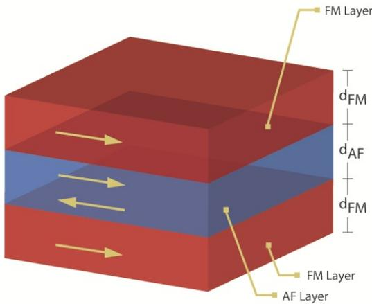
FIGURE 1. System construction. Lower and upper layer correspond to FM phase ( $x=1/3$ ). Intermediate layer correspond to AF phase ( $x=2/3$ ).
