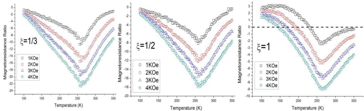
FIGURE 3. %MR as function of Temperature.  $\xi = 1/3$  and  $1/2$  have a regular behavior of magnetoresistance. Applied magnetic field always produces a decrease in the resistivity for all ranges of temperature. On the other hand,  $\xi = 1$  has the special feature that low temperatures increases resistivity and high temperatures present regular MR effect.
