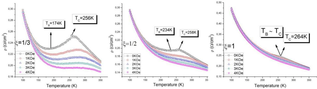
FIGURE 2. Resistivity values as a function of the temperature for several values of magnetic field (0kOe-4kOe) and three values of  $\xi$ . Transition temperature ( $T_C$ ) and blocking temperature ( $T_B$ ) are shown at Zero Field. Different values of external magnetic field change these parameters. When  $\xi = 1$  blocking temperature is overlapped with  $T_C$ .
