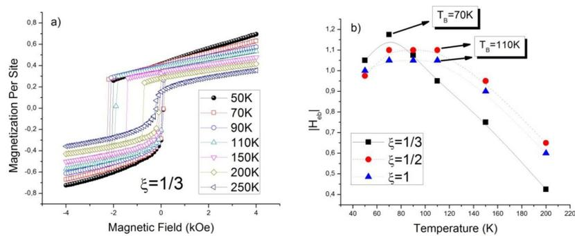
FIGURE 4. a) Hysteresis Loops for different values of Temperatures. Exchange Bias phenomenon is exhibited. b) Variation of the Exchange Field as a function of temperature. In  $\xi = 1/3$ . A lower blocking temperature is exhibited around 70K and when  $\xi$  grows enough, a higher blocking temperature is established around 110K.
