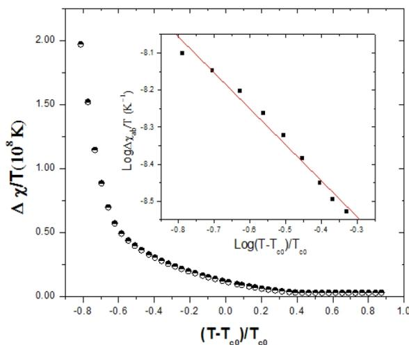
FIGURE 4. Diamagnetism excess as a function of reduced temperature for the  $\text{La}_{0.5}\text{Dy}_{0.5}\text{BaCaCu}_3\text{O}_{7-\delta}$  sample.
