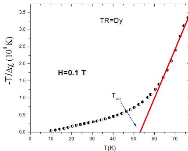
FIGURE 3. Exemplification of experimental method used to find the reduced temperature  $T_{c0}$  in the  $\text{La}_{0.5}\text{Dy}_{0.5}\text{BaCaCu}_3\text{O}_{7-\delta}$  sample.
