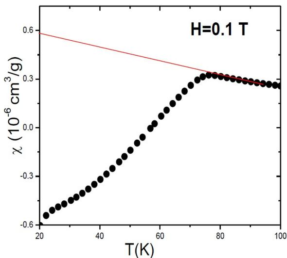
FIGURE 2. Experimental data of magnetic susceptibility for  $\text{La}_{0.5}\text{Dy}_{0.5}\text{BaCaCu}_3\text{O}_{7-\delta}$ .
