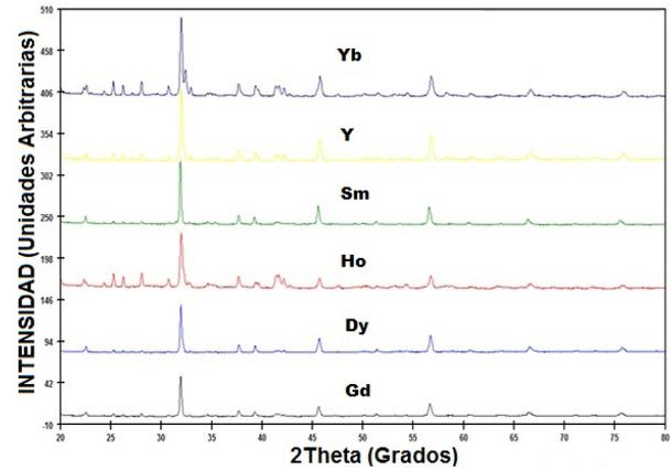
FIGURE 1. XRD spectra for  $\text{La}_{0.5}\text{TR}_{0.5}\text{Ba}_2\text{CaCu}_3\text{O}_{7-\delta}$  (TR = Dy, Gd, Y, Yb, Sm y Ho).
