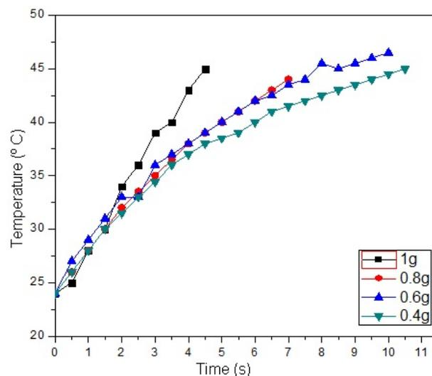
FIGURE 2. Influence of the concentration of magnetic tracers on the time to heat water phantoms to  $45 \text{ }^\circ\text{C}$ .
