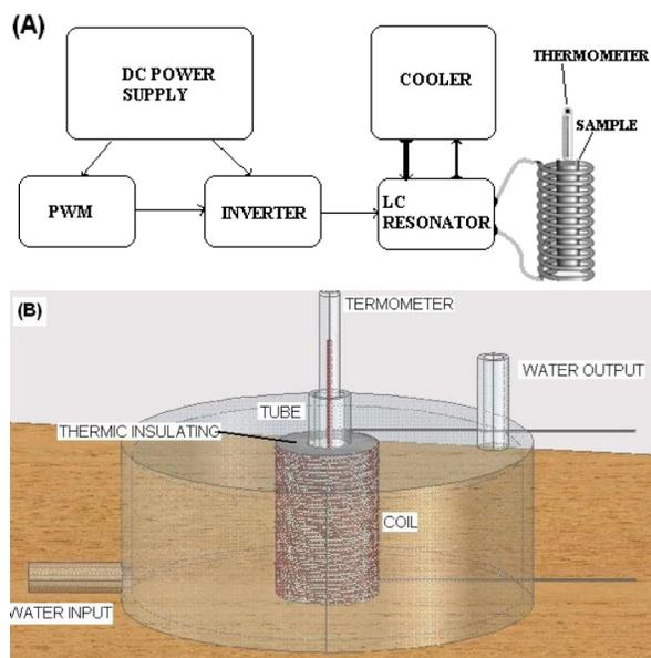
FIGURE 1. Scheme for the general setup of the experiment (A) and of the induction coil with its cooling element (B).
