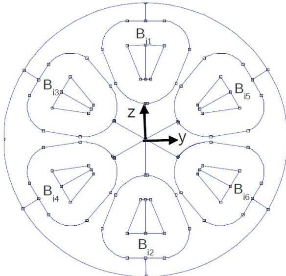
FIGURE 1. Schematic illustration of the arrangement of used pick-up coils.
