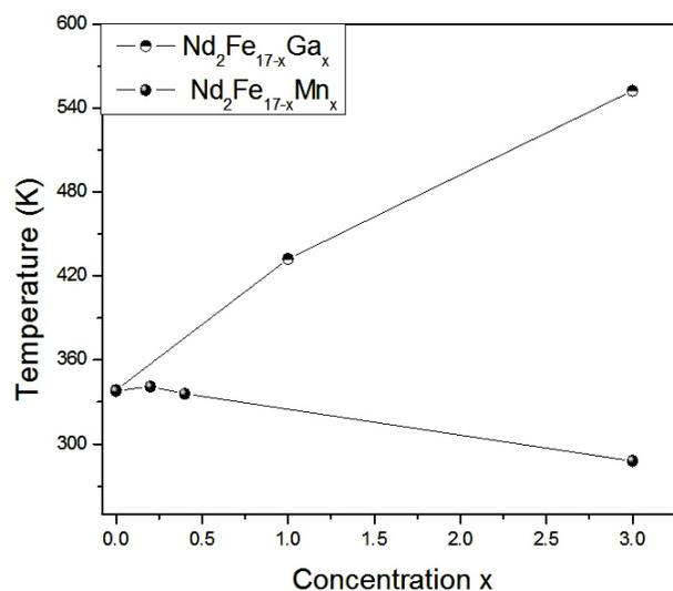
FIGURE 2. Dependence of  $T_c$  with the concentration  $x$  for  $\text{Nd}_2\text{Fe}_{17-x}\text{M}_x$  ( $\text{M} = \text{Ga}, \text{Mn}$ ), measured with MTG.
