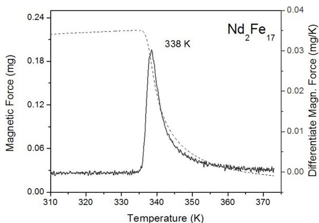
FIGURE 1. Magnetic Force Curve vs Temperature and Differentiate Magnetic Force  $\text{Nd}_2\text{Fe}_{17}$  sample.
