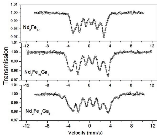
FIGURE 3. Mössbauer Spectra of  $\text{Nd}_2\text{Fe}_{17-x}\text{Ga}_x$  at 300 K
