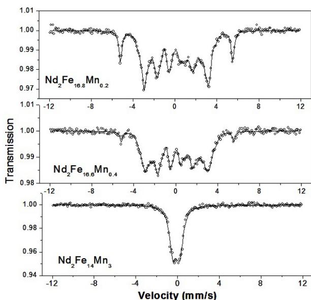
FIGURE 4. Mössbauer Spectrum of  $\text{Nd}_2\text{Fe}_{17-x}\text{Mn}_x$  at 300 K
