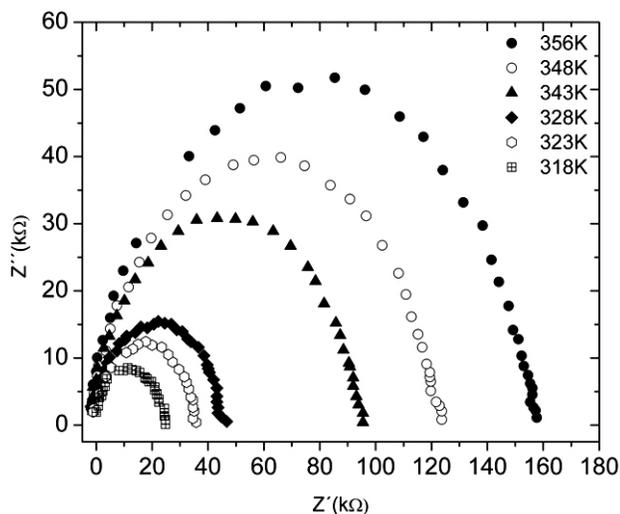
FIGURE 1. Nyquist diagram from impedance measurements for  $\text{Nd}_2\text{Fe}_{16.6}\text{Mn}_{0.4}$ .
