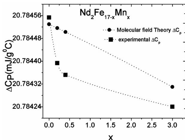
FIGURE 3.  $\Delta C_p$  vs x for Nd<sub>2</sub>Fe<sub>17-x</sub>Mn<sub>x</sub> from experimental data and for an expression derived from molecular field theory, dotted line is a visual guide.
