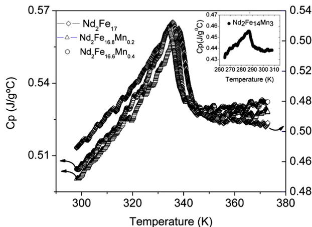
FIGURE 2. Specific heat measurements as functions of temperature near  $T_c$  for  $\text{Nd}_2\text{Fe}_{17-x}\text{Mn}_x$  obtained from MDSC. Left and right scales associate with respective curves as indicated by the arrows.
