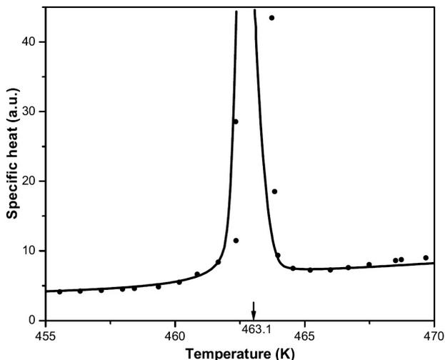
FIGURE 2. Temperature dependence of specific heat  $c_P(T)$  under normal pressure as a function of temperature for an sample of alumel, which shows a sharp peak at  $T_C = 463$  K.
