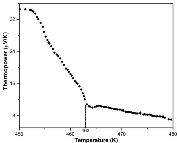
FIGURE 1. Temperature dependence of the thermoelectrical power of alumel close to the ferromagnetic-paramagnetic phase transition.
